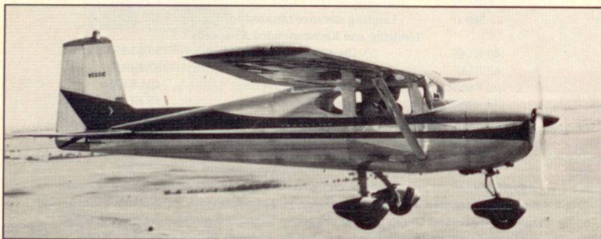
The early 150s are distinguished by their square tails and fastback empennage design.
